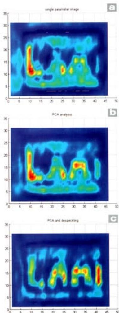
(a) Original mm-wave image of the object (b) image improved with principal component analysis; (c) image improved by means of a despeckling algorithms.
